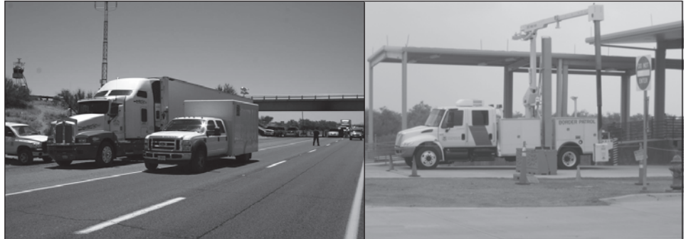
Figure 10: Van with Backscatter X-ray Scanning a Truck (left photograph) and VACIS Unit (right photograph) Used at Checkpoints to Detect Concealed Persons or Contraband
