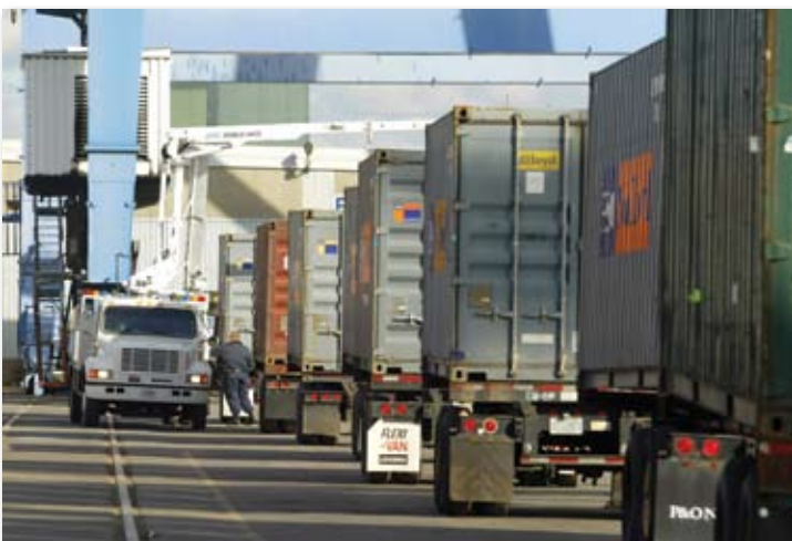
The mobile VACIS employs a gamma ray source to produce images of vehicles for contraband.
